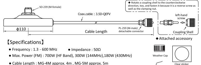
Connector: SO-239 (M-Female) / Magnet base, PL-259 (M-male) / detachable connector
